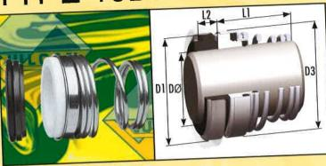
'O'-Ring mounted, conical spring, shaft directional dependent seal, with pressed stainless steel head retainer and 'O'-Ring mounted seal and stationary faces.
